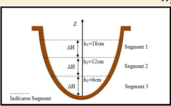
$$K_2 = \frac{t}{A_2 \Delta H} \left(\frac{4V_2}{\Delta T_2} - \frac{16V_3}{\Delta T_3}\right)$$
