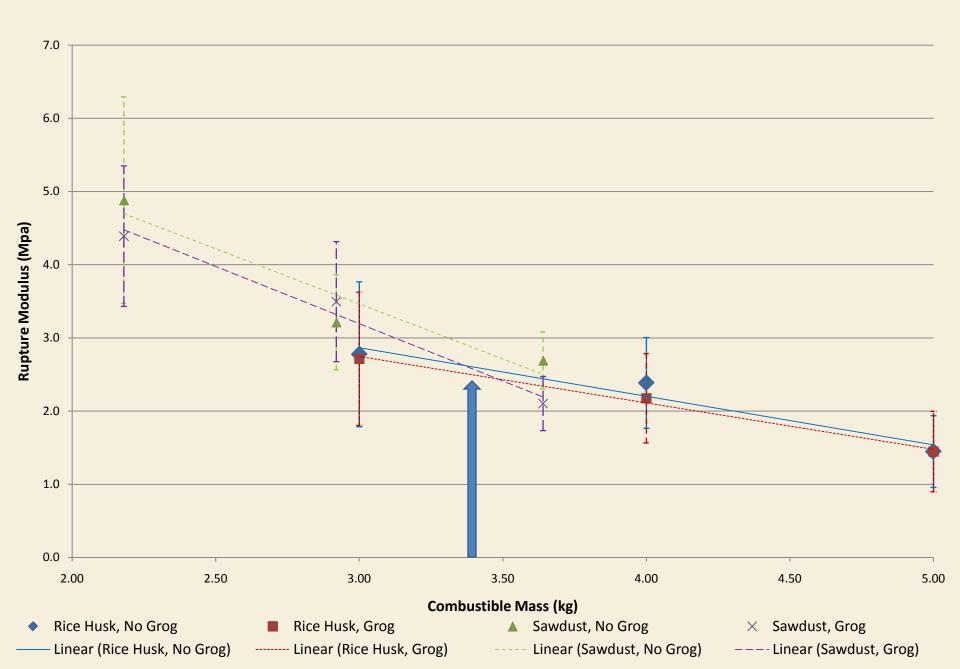
**Comparison of Mean Modulus of Rupture for Recipes Containing Similar Masses of Different Combustible Types, 95% Confidence**
