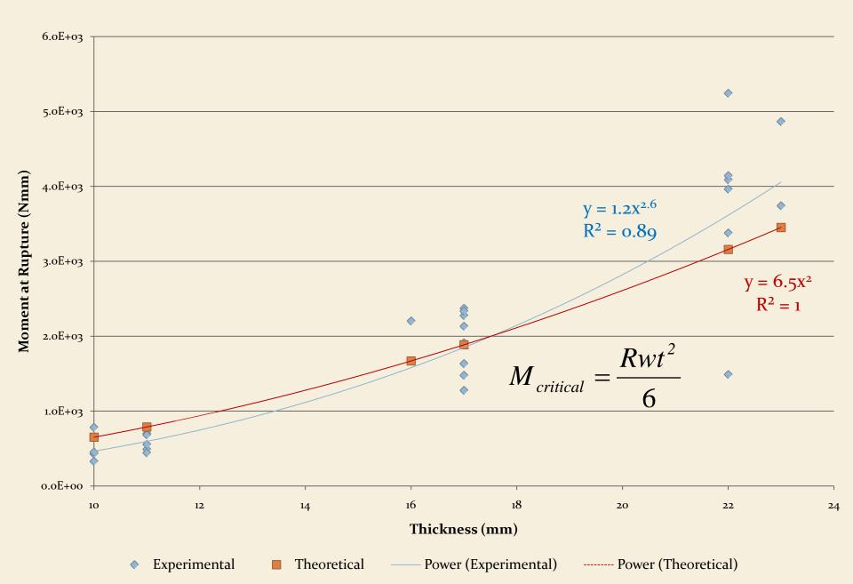
**Comparison of Allowable Moment for Samples of Varying Thickness,** 95% Confidence
