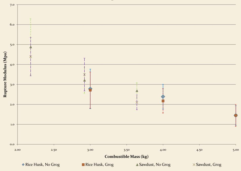
Comparison of Mean Modulus of Rupture Between Recipes with Incrementally Differing Combustible Mass, 95% Confidence
